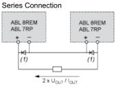
(1) Two Shottky diodes Imin = power supply In and Vmin = 50 V
